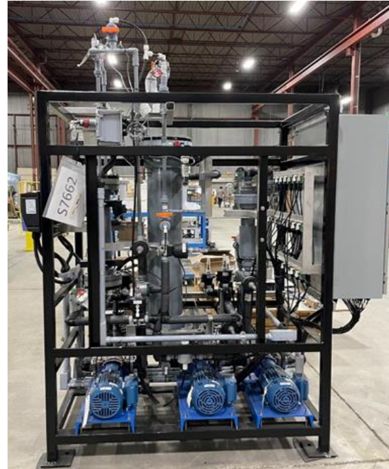
Image: transportable lithium extraction pilot unit by eco-tech, a Koch Separation Solutions Company
