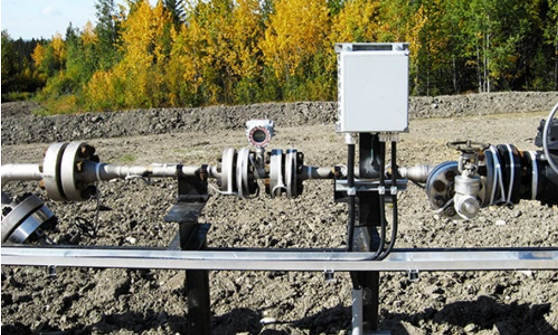
Figure 18-3: Pipeline Flow Measurement and Leak Detection System
